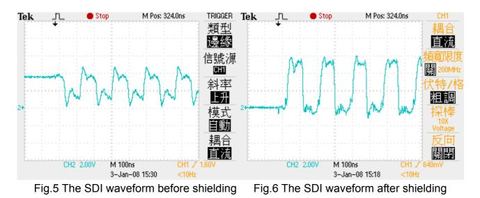
3. When the signal is bounced from the receiver end to the transmitter end, the superposed signal disturbs the internal function of the CS8803. To prevent the
