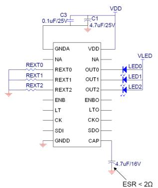
Fig.2 Connecting CAP with adequate capacitor to stabilize the signal
